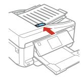
Note: If you're using the Letter, 2-up Copy, or A4, 2-up Copy layout, make sure the originals are loaded as shown.
